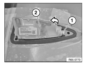
If necessary, release screw (1) and raise multiband telephone antenna (2).
