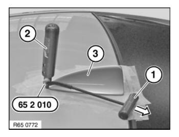
Cut through adhesive bead all round with special tool  $\underline{65\ 2\ 010}$  .
