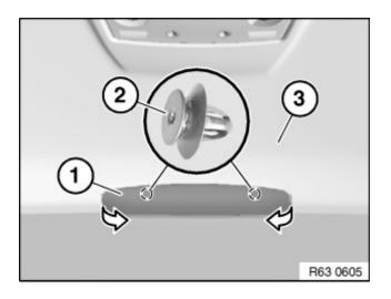
Unclip cover for additional brake light (1) at points (2) and feed out sideways in direction of arrow.
